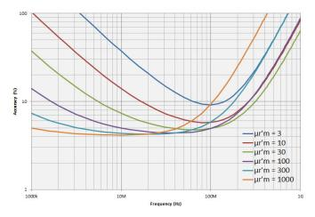
Figure 45. Permeability accuracy  $(\Delta \mu'_r)$  vs. frequency (at F = 0.5 mm, typical)  $\mu'_r$
