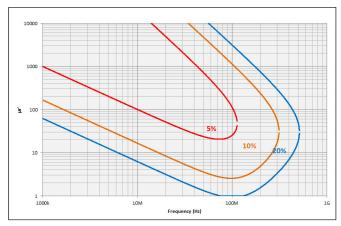
Figure 28. Permeability  $(\mu'_r)$  vs. frequency (at F = 0.5 mm, typical)
