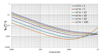
Figure 55. Typical frequency characteristics of temperature coefficient of  $\epsilon'_{\rm r}$  (Thickness = 1 mm)
