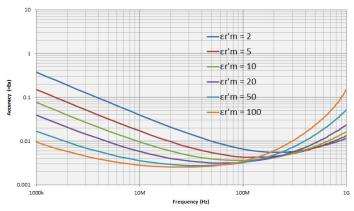
Figure 39. Dielectric loss tangent (tan $\delta$ ) accuracy vs. frequency (at t = 0.3 mm, typical) <sup>1</sup>
