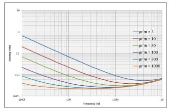
Figure 25. Permeability loss tangent (tan $\delta$ ) accuracy vs. frequency (at F = 0.5 mm, typical) <sup>1</sup>
