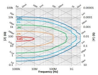
Figure 31. [Z], [Y] measurement accuracy when open/short/load calibration is performed. Oscillator level = -13 dBm, -3 dBm. Point averaging factor  $\geq 8$  within  $\pm 5 \text{ °C}$  of calibration temperature.
