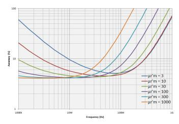
Figure 46. Permeability accuracy  $\left(\frac{\Delta \mu_{i}^{t}}{\mu_{r}^{t}}\right)$  vs. frequency (at *F* = 3 mm, typical)
