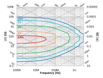
Figure 3. [Z], [Y] Measurement accuracy when open/short/load calibration is performed. Oscillator level = -33 dBm. Point averaging factor  $\ge 8$  within  $\pm 5$  °C from the calibration temperature.
