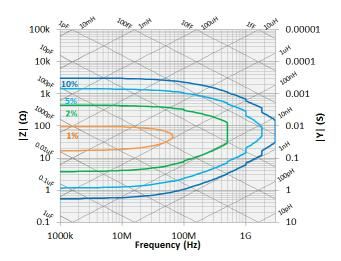
Figure 34. |Z|, |Y| measurement accuracy when open/short/load calibration is performed. Oscillator level = -33 dBm. Point averaging factor  $\leq 7$  within  $\pm 5$  °C of calibration temperature.
