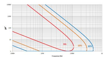
Figure 53. Permeability  $(\mu'_r)$  vs. frequency (at F = 10 mm, typical)
