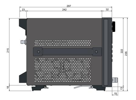
Figure 9. Main unit dimensions (side view, in millimeters).
