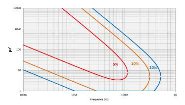
Figure 52. Permeability  $(\mu'_r)$  vs. frequency (at F = 3 mm, typical)
