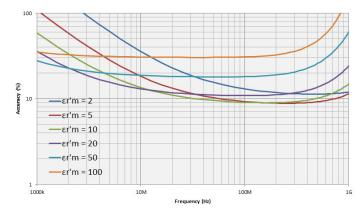
Figure 37. Permittivity accuracy  $(\frac{\Delta \mathbf{\hat{\epsilon}}'}{\mathbf{\hat{\epsilon}}'_{t}})$  vs. frequency, (at t = 1 mm typical)
