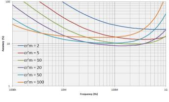
Figure 38. Permittivity accuracy  $(\frac{\Delta \varepsilon'}{\varepsilon'_{r}})$  vs. frequency, (at t = 3 mm typical)
