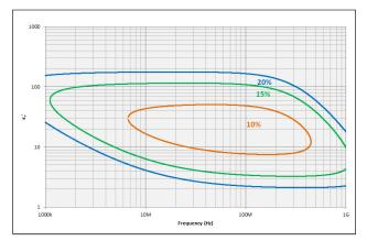
Figure 21. Permittivity (['<sub>r</sub>) vs. frequency (at t = 3 mm, typical)
