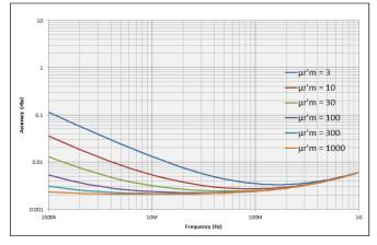
Figure 26. Permeability loss tangent (tan $\delta$ ) accuracy vs. frequency (at *F* = 3 mm, typical)<sup>1</sup>
