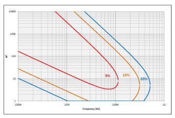
Figure 29. Permeability  $(\mu'_r)$  vs. frequency (at F = 3 mm, typical)
