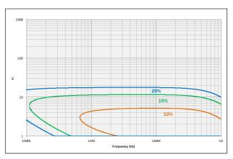
Figure 19. Permittivity ([' $_r$ ) vs. frequency (at t = 0.3 mm, typical)
