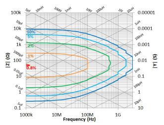
Figure 32. |Z|, |Y| measurement accuracy when open/short/load calibration is performed. Oscillator level –13 dBm, –3 dBm. Point averaging factor  $\leq$  7 within ± 5 °C of calibration temperature.
