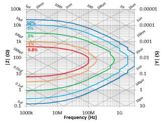
Figure 2. |Z|, |Y| Measurement accuracy when open/short/load calibration is performed. Oscillator level –13 dBm, –3 dBm. Point averaging factor  $\leq$  7 within ± 5 °C from the calibration temperature.
