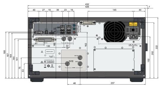
Figure 8. Main unit dimensions (rear view, in millimeters).
