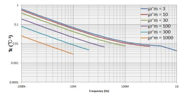
Figure 57. Typical frequency characteristics of temperature coefficient of  $\mu'_{c}$  (at F = 0.5 mm)
