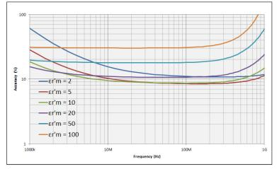
Figure 14. Permittivity accuracy  $(\frac{\Delta \mathbf{\tilde{e}'}_r}{\mathbf{\tilde{e}'}_r})$  vs. frequency (at t = 1 mm, typical).
