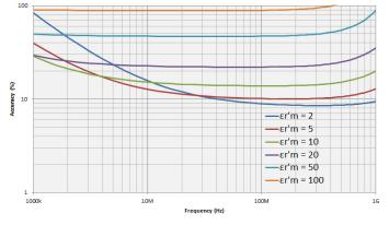
Figure 36. Permittivity accuracy  $(\frac{\Delta \varepsilon'}{\varepsilon'_r})$  vs. frequency, (at t = 0.3 mm typical)
