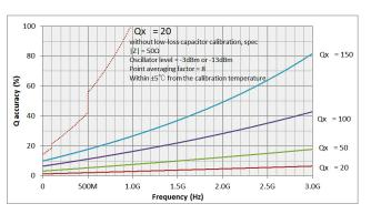
Figure 5. Q accuracy without low-loss capacitor calibration (Specification) and with low-loss capacitor calibration (Typical).
