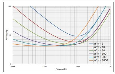
Figure 22. Permeability accuracy  $\left(\frac{\Delta \mu'}{\mu'_r}\right)$  vs. frequency (at F = 0.5 mm, typical)
