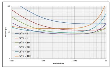
Figure 15. Permittivity accuracy  $(\frac{\Delta \varepsilon' r}{\varepsilon' r})$  vs. frequency (at t = 3 mm, typical).
