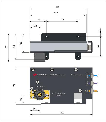
Figure 12. Option E4991B-010 test head dimensions (in millimeters).
