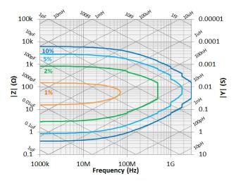
Figure 33. |Z|, |Y| measurement accuracy when open/short/load calibration is performed. Oscillator level = -33 dBm. Point averaging factor  $\ge 8$  within  $\pm 5$  °C of calibration temperature.
