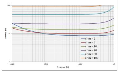
Figure 13. Permittivity accuracy  $(\frac{\Delta \varepsilon' r}{\varepsilon' r})$  vs. frequency (at t = 0.3 mm, typical).
