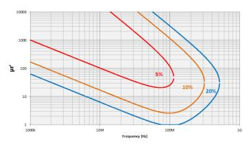
Figure 51. Permeability  $(\mu'_r)$  vs. frequency (at F = 0.5 mm, typical)
