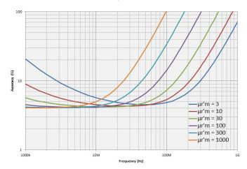
Figure 47. Permeability accuracy  $\left(\frac{\Delta \mu_{f}}{\mu_{e}^{t}}\right)$  vs. frequency (at *F* = 10 mm, typical)
