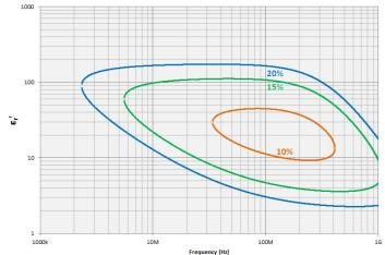
Figure 44. Permittivity  $(\mathbf{\epsilon}'_r)$  vs. frequency (at t = 3 mm, typical)
