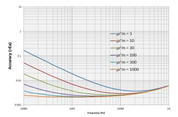
Figure 50. Permeability loss tangent (tan $\boldsymbol{\delta}$ ) accuracy vs. Frequency (at *F* = 10 mm, typical)<sup>1</sup>
