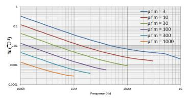
Figure 59. Typical frequency characteristics of temperature coefficient of  $\mu'_{e}$  (at F = 10 mm)
