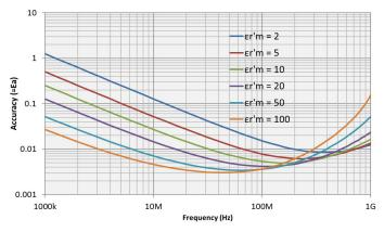
Figure 40. Dielectric loss tangent (tan $\delta$ ) accuracy vs. frequency (at t = 1 mm, typical) <sup>1</sup>
