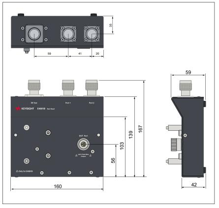
Figure 10. Test head dimensions (in millimeters).
