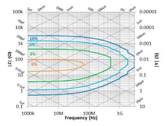
Figure 4. |Z|, |Y| Measurement accuracy when open/short/load calibration is performed. Oscillator level = -33 dBm. Point averaging factor  $\leq$  7 within ± 5 °C from the calibration temperature.
