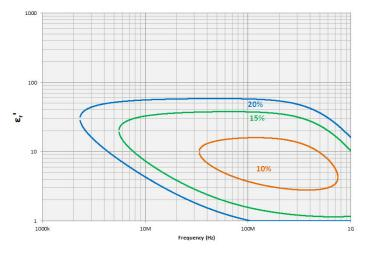
Figure 43. Permittivity ( $\boldsymbol{\epsilon}'_{r}$ ) vs. frequency (at t = 1 mm, typical)
