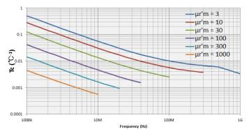
Figure 58. Typical frequency characteristics of temperature coefficient of  $\mu'_c$  (at F = 3 mm)
