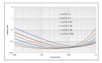
Figure 16. Dielectric loss tangent (tan $\mathbf{\delta}$ ) accuracy vs. frequency (at t = 0.3 mm, typical) <sup>1</sup>
