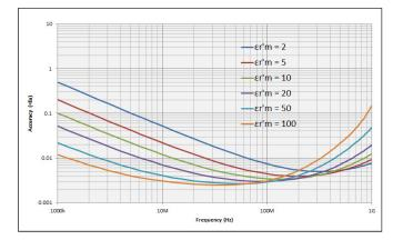
Figure 17. Dielectric loss tangent (tan $\mathbf{\delta}$ ) accuracy vs. frequency (at t = 1 mm, typical) <sup>1</sup>
