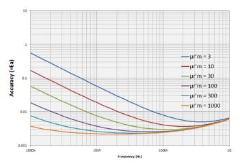
Figure 49. Permeability loss tangent (tan $\delta$ ) accuracy vs. frequency (at F = 3 mm, typical)<sup>1</sup>
