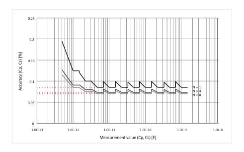
**Figure 9.** Accuracy of Cp and Cs when measurement frequency is 1 MHz (measurement signal level: 1 V)
