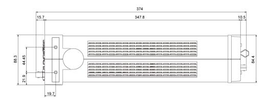
Figure 20. Dimensions (side view, without handle and bumper, in millimeters, nominal)
