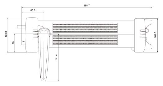
Figure 19. Dimensions (side view, with handle and bumper, in millimeters, nominal)
