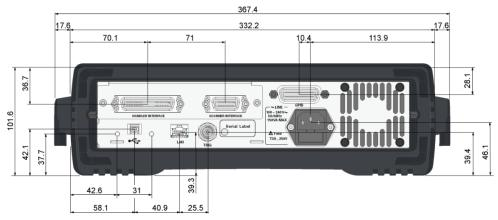
Figure 17. Dimensions (rear view, with handle and bumper, in millimeters, nominal)
