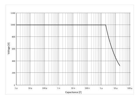
Figure 14. Maximum discharge withstands voltage (typical)
