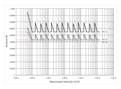
**Figure 1.** Accuracy of D when measurement frequency is 120 Hz (measurement range: 10 nF to 100  $\mu$ F / measurement signal level: 0.5 V)
