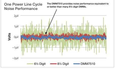
Comparison of the DMM7510's 1 VDC noise performance with that of typical 6%- and 8%-digit multimeters. All data was taken at 1 NPLC with a low thermal short applied to the input.
