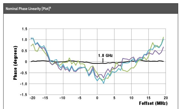
The phase characteristics of analysis frequencies below 3.6 GHz are similar to the 1.8 GHz graph shown. For analysis above 3.6 GHz, the curves shown are representative. They were measured between 5 and 25 GHz. The phase linearity of the analyzer does not depend on the frequency option.
