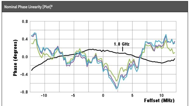
The phase characteristics of analysis frequencies below 3.6 GHz are similar to the 1.8 GHz graph shown. For analysis above 3.6 GHz, the curves shown are representative. They were measured between 5 and 25 GHz. The phase linearity of the analyzer does not depend on the frequency option.
