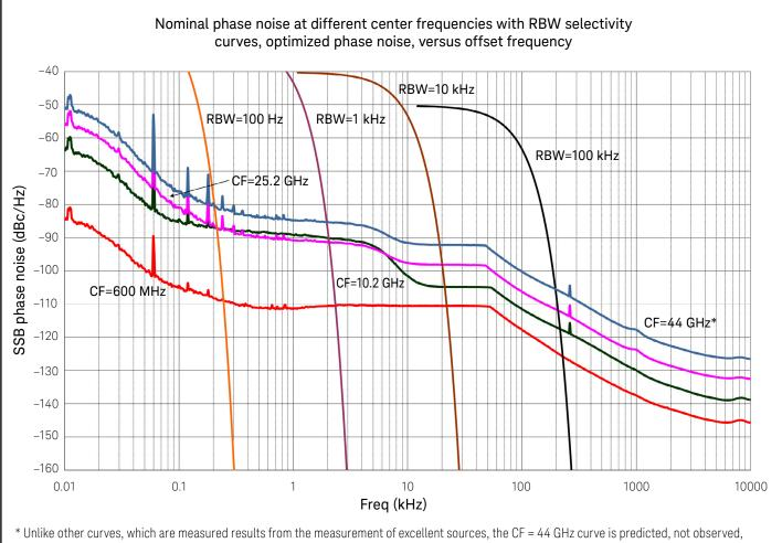
phase noise computed from the 25.2 GHz observation. See the Frequency Stability section for the details of phase noise performance versus CF.
