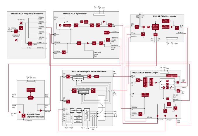
**Figure 2.** Block diagram for a 44 GHz signal generator (M9383A-F44) with 1 GHz bandwidth and enhanced phase noise.
