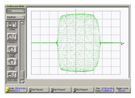
**Figure 3.** Measured pulse shape; Frequency = 9 GHz, power = 5 dBm, amplitude = 5 dBm, ALC off, pulse width = 50 ns, pulse period = 200 ns. The oscilloscope is protected by a 10 dB pad and the timescale is set to 10 ns/div.
