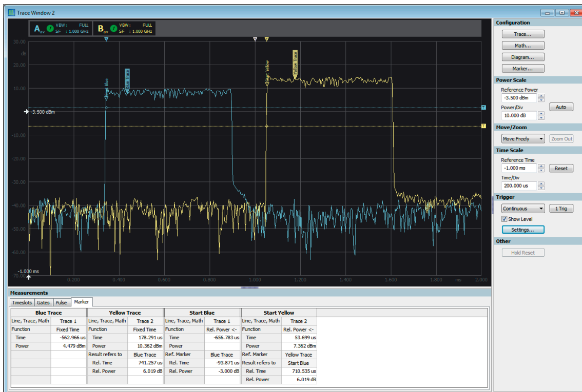
Pulse delay measurement on different traces
