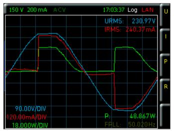
Waveform function: load with phase-angle control
