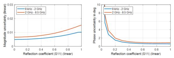
Uncertainty of reflection magnitude and reflection phase measurements for the R&S <sup>®</sup>ZNBT8 in the frequency range from 9 kHz to 8.5 GHz; analysis conditions:  $S_{12} = S_{21} = 0$ , calibrated power – 10 dBm, measured power – 10 dBm
