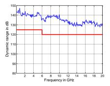
Measured dynamic range in dB versus frequency for the R&S<sup>®</sup>ZNBT20
