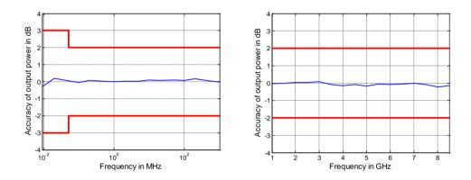
Measured output power accuracy in dB versus frequency for the R&S<sup>®</sup>ZNBT8
