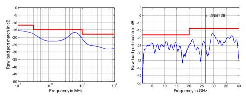
Measured raw load port match versus frequency for the R&S®ZNBT26 and R&S®ZNBT40
