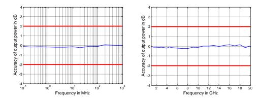
Measured output power accuracy in dB versus frequency for the R&S<sup>®</sup>ZNBT20
