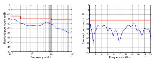
Measured raw load port match versus frequency for the R&S®ZNBT20
