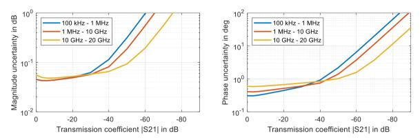
Uncertainty of transmission magnitude and transmission phase measurements for the R&S<sup>®</sup>ZNBT20 in the frequency range from 100 kHz to 20 GHz; analysis conditions:  $S_{11} = S_{22} = 0$ , calibrated power – 10 dBm, measured power – 10 dBm
