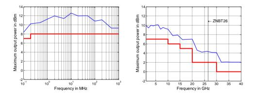
Measured maximum output power in dBm versus frequency for the R&S®ZNBT26 and R&S®ZNBT40
