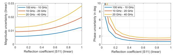
Uncertainty of reflection magnitude and reflection phase measurements for the R&S<sup>®</sup>ZNBT26 and R&S<sup>®</sup>ZNBT40 in the frequency range from 100 kHz to 40 GHz; analysis conditions:  $S_{11} = S_{22} = 0$ , calibrated power –10 dBm, measured power –10 dBm
