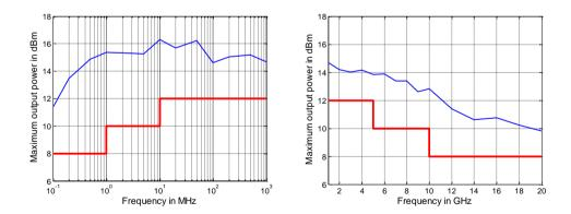
Measured maximum output power in dBm versus frequency for the R&S®ZNBT20
