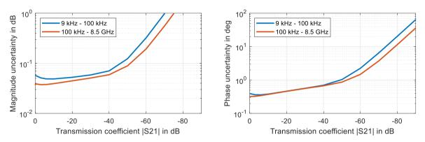
Uncertainty of transmission magnitude and transmission phase measurements for the R&S<sup>®</sup>ZNBT8 in the frequency range from 9 kHz to 8.5 GHz; analysis conditions:  $S_{11} = S_{22} = 0$ , calibrated power –10 dBm, measured power –10 dBm
