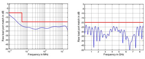
Measured raw load port match versus frequency for the R&S®ZNBT8
