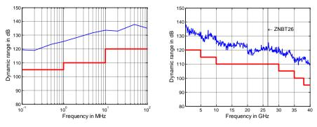
Measured dynamic range in dB versus frequency for the R&S<sup>®</sup>ZNBT26/R&S<sup>®</sup>ZNBT40
