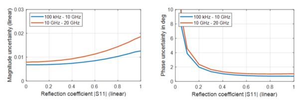
Uncertainty of reflection magnitude and reflection phase measurements for the R&S<sup>®</sup>ZNBT20 in the frequency range from 100 kHz to 20 GHz; analysis conditions:  $S_{12} = S_{21} = 0$ , calibrated power –10 dBm, measured power –10 dBm
