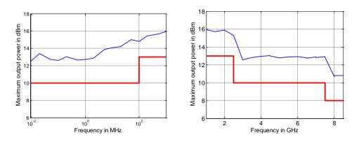
Measured maximum output power in dBm versus frequency for the R&S®ZNBT8
