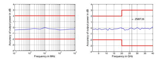
Measured output power accuracy in dB versus frequency for the R&S®ZNBT26 and R&S®ZNBT40
