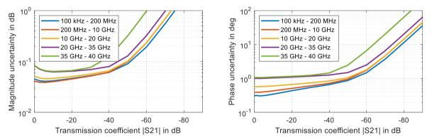
Uncertainty of transmission magnitude and transmission phase measurements for the R&S<sup>®</sup>ZNBT26 and R&S<sup>®</sup>ZNBT40 in the frequency range from 100 kHz to 40 GHz; analysis conditions:  $S_{11} = S_{22} = 0$ , calibrated power –10 dBm, measured power –10 dBm
