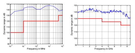
Measured dynamic range in dB versus frequency for the R&S<sup>®</sup>ZNBT8
